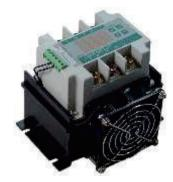
Model: SCR-51-3428 40 amps overall size:118mm\*140mm\*118mm Mounting size:55mm\*135mm
