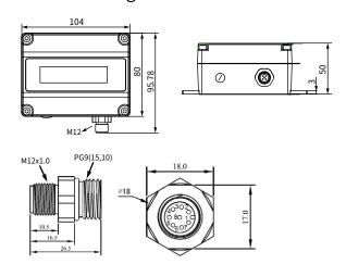
2.N type: M16-8PIN metal connector (RS-485+analog)
