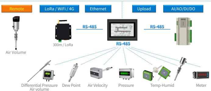
eYc AIOT Solution - System Architecture of the Smart Factory
