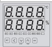
INDICATOR OUT: The flashing frequency indicate the output ratio
