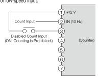
2. In the case of no-contact input signals
