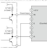
When used as shown in the figure below, the voltage and current that flow through the contact point are around 2 mA. Therefore, the use of the contact point for minute electric current improves reliability. Since the contact point of the electromagnetic switch is designed for large current and high voltage, it is not suitable for use for contact input of the counter.
