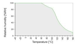
The grey area shows the allowed measurement range for the humidity sensor.
