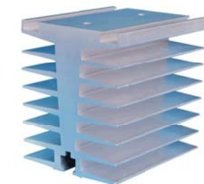
Model: MW-T-80 Size: 80mm*80mm*70mm For 80amps,100amps,120amps Mounting method: Panel mount or din rail mount with din rail adaptor
