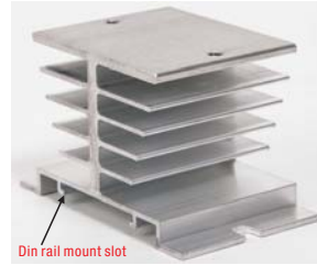
Model: MW-I-50 Size: 60mm*50mm*50mm For 10 amps/25 amps SSR Mounting method: Panel mount or din rail mount directly
